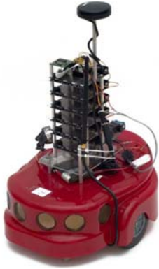
Fig. 5 – Experimental Testbed. Clusters of these vehicles were controlled using the cluster space technique. On-board equipment includes GPS, a compass, and an array of microcontrollers. A GUI allows an operator to directly specify and monitor the motion of the two-robot cluster in real-time.
