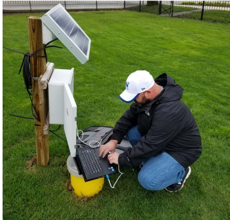
Monitoring a solar powered instrument well of a geothermal project at Ball State University. Photo credit: BSU CERES
